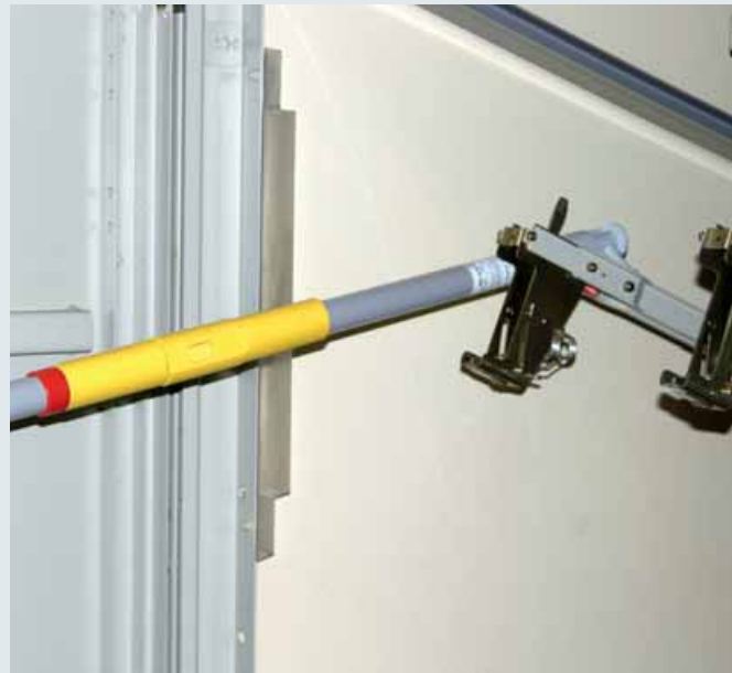
IS STK insulating stick fitted with STK switching stick head used as switching stick
